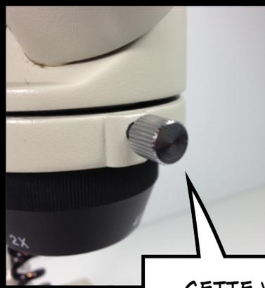
CETTE VIS PERMET DE FIXER LA TÊTE DU BINO. ON LA MAINTIENS TOUJOURS VISSÉE, SAUF LORSQU'ON FAIT TOURNER LA TÊTE DU BINO.
