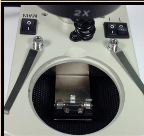
IL Y A UNE AMPOULE SOUS LA PLAQUE OPTIQUE. AVEC LA PLAQUE TRANSLUCIDE, ON L'UTILISE POUR VOIR EN TRANSPARENCE.
