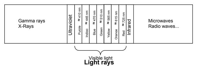
Like all electromagnetic waves, light travels in straight lines in a vacuum. In a classroom where temperature is stable, we can consider that light will travel in a straight line. In class, we will call light that travels in a straight line "light rays" or "rays of light".
