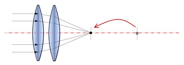
• The addition of a slightly divergent lens makes the rays converge more slowly. This distances the focal point from the lenses.
