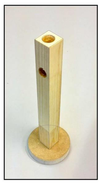
It is possible to supply a stand on which to test the students' wheels. The model shown at left is one suggestion. It is made from a 1" X 9.5" wooden moulding, in which we drilled two holes with a diameter of 5/8". The moulding is screwed into a base, which may be round or square.
