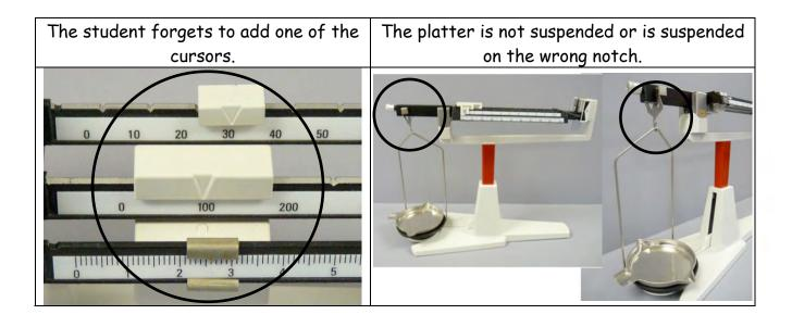
Check that the platter #, platter support # and the scale # are identical, because the scale is calibrated in relation to each part.
