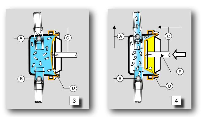
Initially, the deformation of the membrane causes the expulsion of air by the upper valve. When the membrane turns to its original position, the vacuum created causes a depression which aspirates the water (opening the bottom valve) in the cavity (container).
