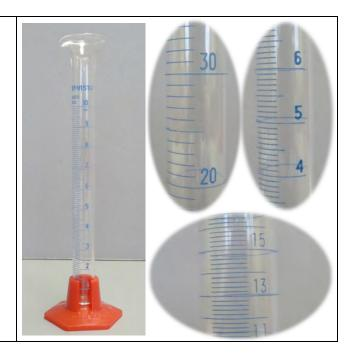
2- I carefully pour the liquid to be measured into the cylinder.
