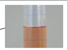
5- Using a transfer pipette or a dropper, I add or remove liquid as necessary.
