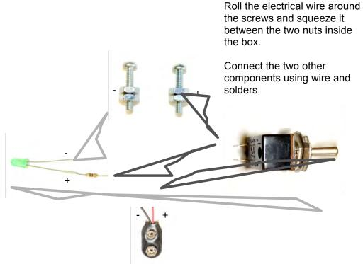
3- Install the battery in the housing using self-adhesive Velcro and connect it to the circuit using the connector.
