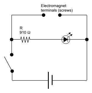
1- Solder the LED anode (positive electrode) to one of the legs of the resistor.
